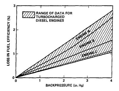
FIG. 28. RELATIONSHIP OF DIESEL ENGINE FUEL EFFICIENCY TO EXHAUST BACKPRESSURE.
