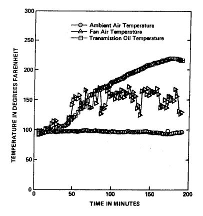
FIG. 26. TEMPERATURE TESTS OF FORD CLT 9000 WITH ACOUSTICAL PANELS.
